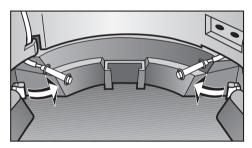
■ To remove the drip tray, begin by carefully unclipping the water sensors, then bend them gently upward.
